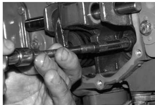
**Second from bottom: with the valve stem hanging out the plug hole, it may be cleaned of deposits...and (above) a reamer may be gently used to clean deposits from the guide.**
