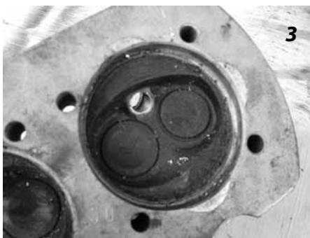
Top: lubricate the threads of the spark plug and wind it in by hand; Above, get the torque spec for your engine and use a torque wrench to tighten. All done.
