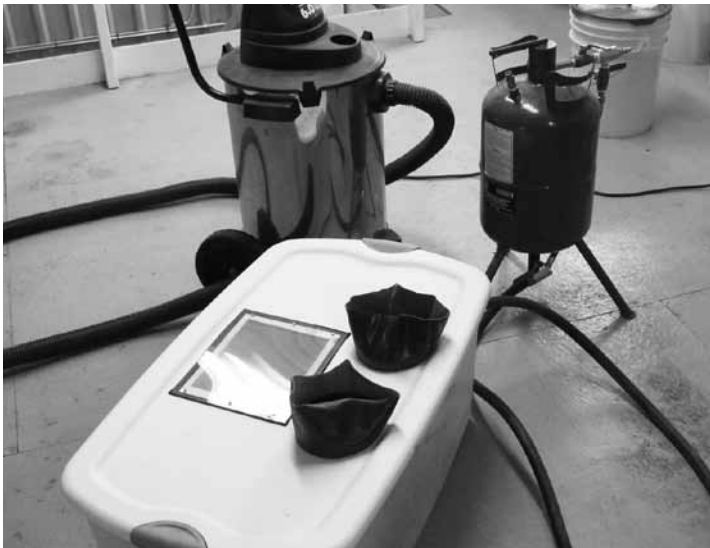
The whole shebang: the $25 dollar cabinet with the necessary appendages: a shop vac and some compressed air.
