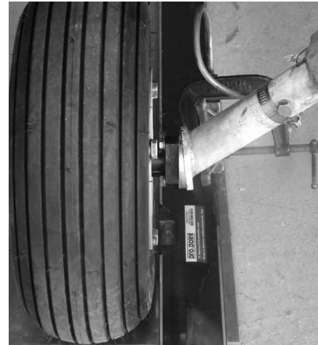
Above left: My Rocket has a tapered aluminum spacer between the gearleg and the bolt on axle. I was lucky that by rotating I could use the same spacer. Otherwise I would have been off to Spruce or to a friend's machine shop for a custom part. Right: Camber can be checked with a framing square. The grease plates have moved quite a lot during the iterations of the test. If they pick up grit they will stop sliding, so keep the floor clean
