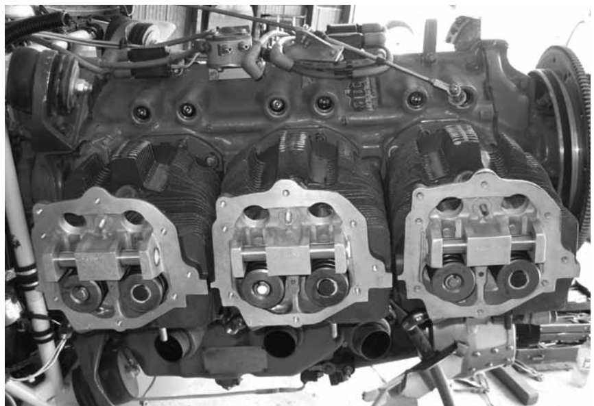
From the top down: Installing cylinder and piston on the connection rod; Removing the piston pin; The cylinders in place
