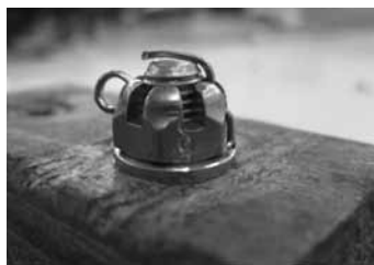
Fig. 2 (Correct Cotter Pin Installation)
