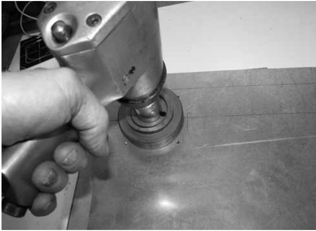
Left, Updrill to 5/8 with a step drill and use the ATS punch for the panel hole. A pneumatic wrench makes this easy. Right, try to avoid anything that looks like this
