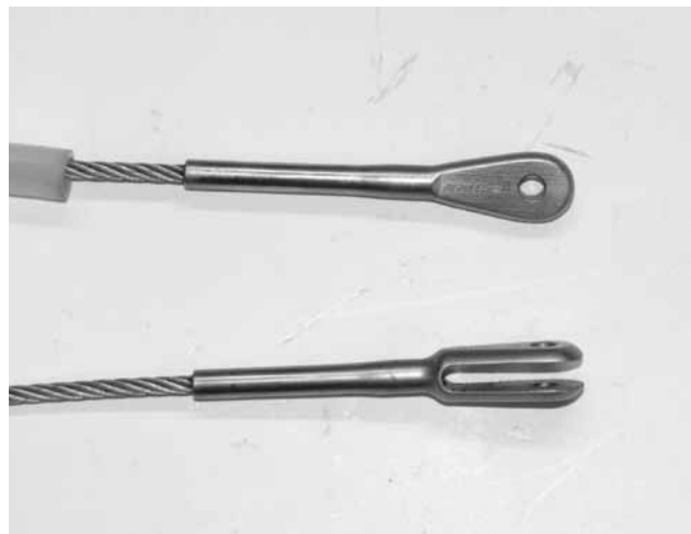
Left: For the second end, if another set of hands is not available, a cleco clamp can help to hold the cable. Right: Here are typical cable ends that Spruce will fit to order, +/- 1/8" length tolerance
