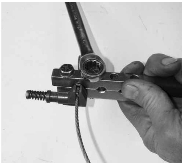
Left: For the second end, if another set of hands is not available, a cleco clamp can help to hold the cable. Right: Here are typical cable ends that Spruce will fit to order, +/- 1/8" length tolerance
