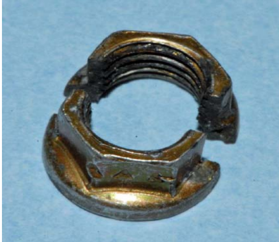
Figure 1 above illustrates a failed nut found by an operator that had split in two.
