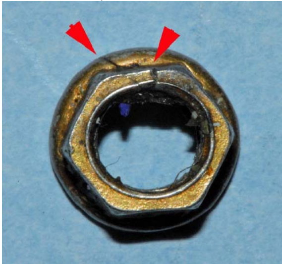
Figure 2 indicates a typical finding of a cracked nut.
